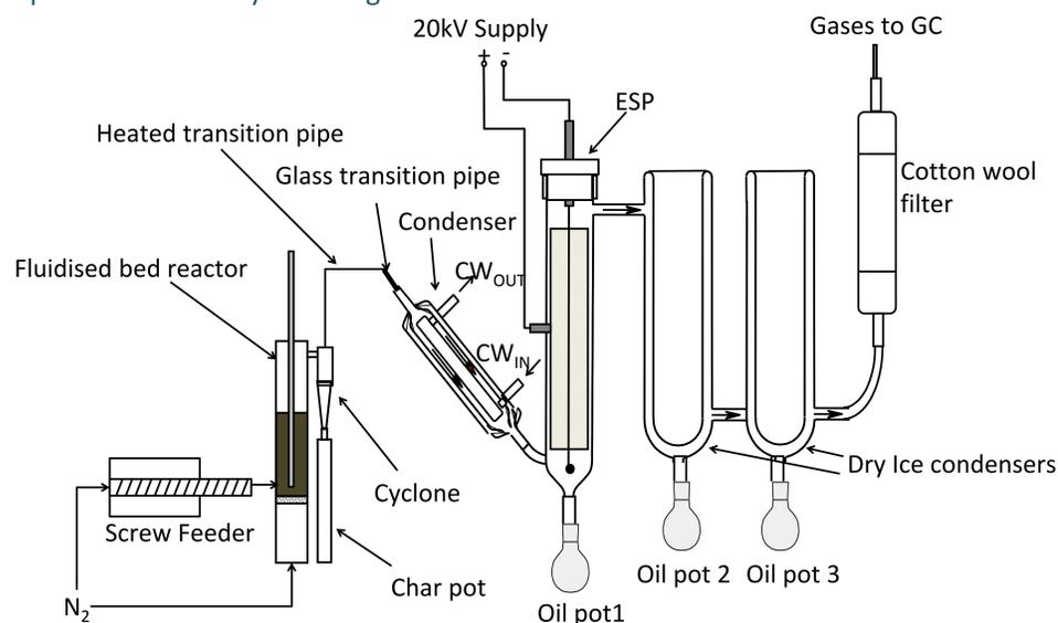
Figure 2. Continuous fluidised bed fast pyrolysis system
