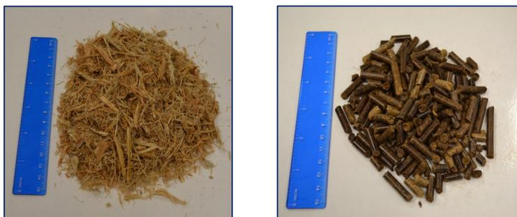
Figure 1. Sugarcane bagasse (left) Sugarcane bagasse pellets (right)
