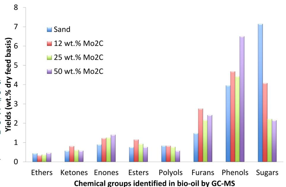
Figure 3. Effect of  $\text{Mo}_2\text{C}/\text{Al}_2\text{O}_3$  concentration on bio-oil composition
